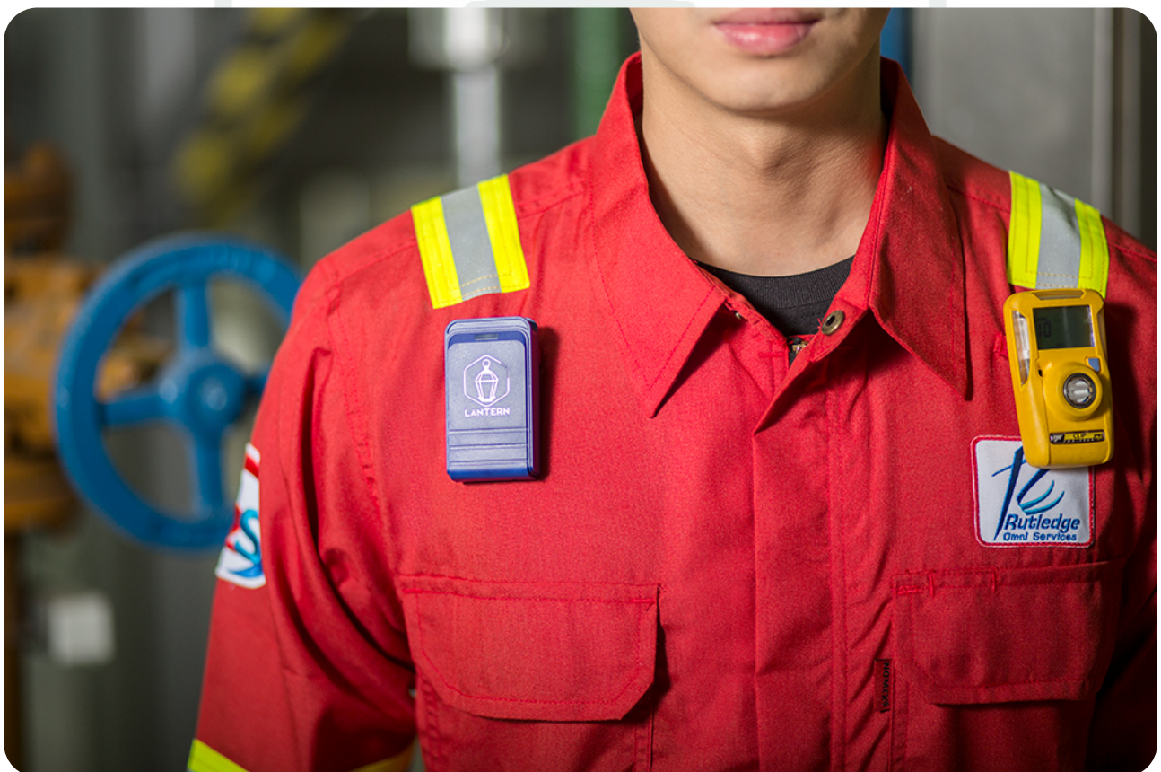
The Lantern Tag is a wearable device designed to withstand harsh industrial conditions
